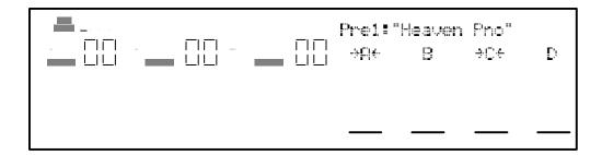
All MIDI channels that are active in the current Mix are shown at the top left, to indicate multitimbral operation. The current MIX and EFFECT numbers are displayed, along with the current Bank and Mix's name. The PROGram number display shows the program assigned to the <u>underlined</u> MIDI channel.
