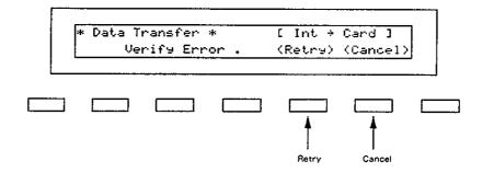
To transfer the data from the Memory Card again, assign RETRY with the Selector Button and repeat the transfer procedure after carefully reading the instructions of the Memory Card.
