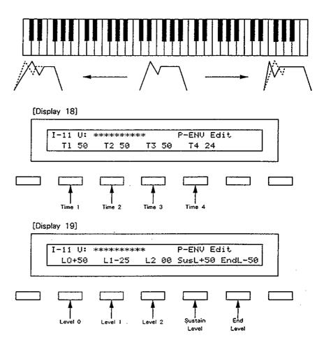
The envelope curve is determined by times and levels.
