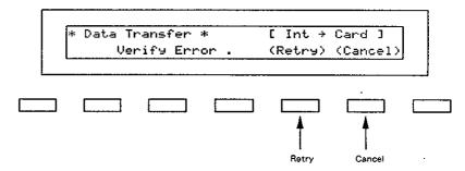
To transfer the data onto the Memory Card again, assign RETRY with the Selector Button and repeat the transfer procedure after carefully reading the instructions of the Memory Card.
