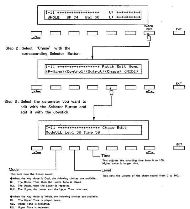
\*Depending on the Chase Level and Velocity, the number of repeats of the delayed sound differ, If "TVA Velocity Sens" (page 43) is set to 0, the sound does not decay but repeats with the same time.
