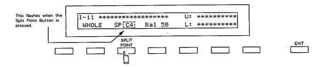
Step 2 Using the Joystick, set the Split Point represented by a note name..
