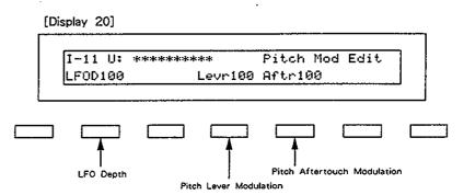
\*Depending on how the LFO in WG modulation (Display 27) is set, the vibrato set here may have no effect at all. Higher values deepen the effect.
