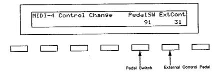
The external MIDI device can be controlled with the pedal switch or external control pedal.
