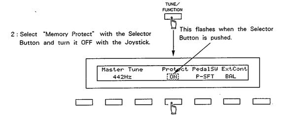
◆To write the data onto the optional Memory Card (M-256D), set the Protect Switch of the Memory Card to OFF as follows.
