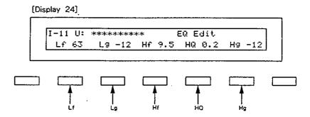
In the equalizer section, the frequency characteristic of the sound can be modified.
