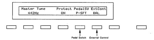
Pushing the button will cause the function currently assigned to the pedal to flash.
