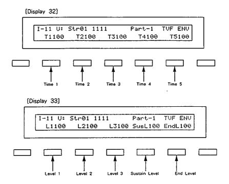
An envelope curve is determined by times and levels.
