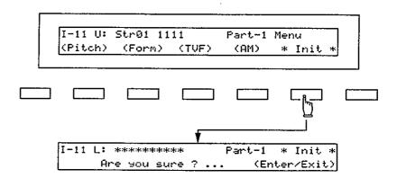
Step 2 Push the Enter Key, and all the parameters of the selected Partial will be initialized, the Display will show as below for a few seconds.
