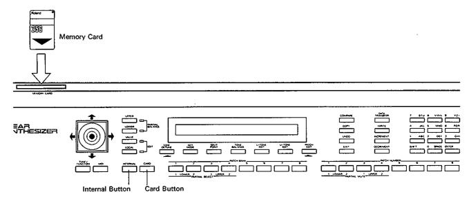
To call a Patch on the Memory Card, simply push the Card Button. To return to the Internal Memory mode, push the Internal Button.
