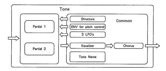
Each Partial (Partial 1 and Partial 2) can have one of two sound generators (a Synthesizer sound source or a PCM sound source). So you can think of the D-50 having powerful synthesizers built in. Each of these hypothetical synthesizers could behave like a conventional analog synthesizer, or a PCM sampled synthesizer. Any combination of two synthesizers can achieve some remarkable cross—modulation effects, so characteristic of today's purely digital sounds.
