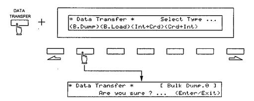
step 6 Push the Enter Key on the transmitter, and the data is transferred,
