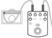
Plug the cable from the OUT jack of the TM-01 to the IN jack of the amplifier.
