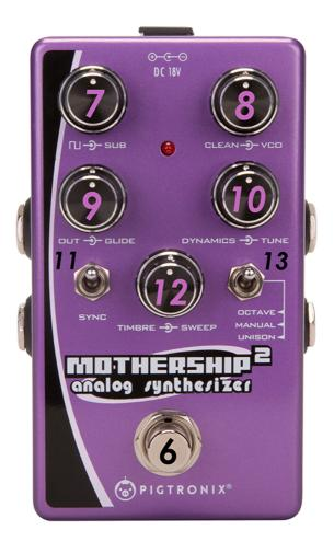
ENGAGE - This footswitch turns the entire Mothership 2 on and off. When the engage light is turned on, the Mothership 2 is active. The Mothership 2 is a true bypass pedal.
